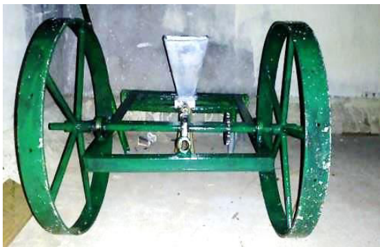
Figure.5 Developed test rig for the analysis of reciprocating seed metering mechanism for groundnut
