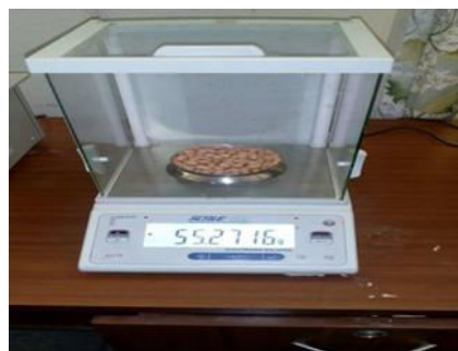
Figure.1 Measuring the physical characteristics of groundnut seeds
