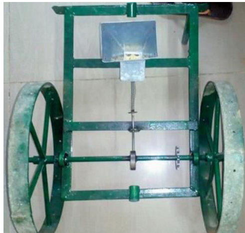
Figure.5 Developed test rig for the analysis of reciprocating seed metering mechanism for groundnut
