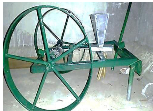
Figure.5 Developed test rig for the analysis of reciprocating seed metering mechanism for groundnut
